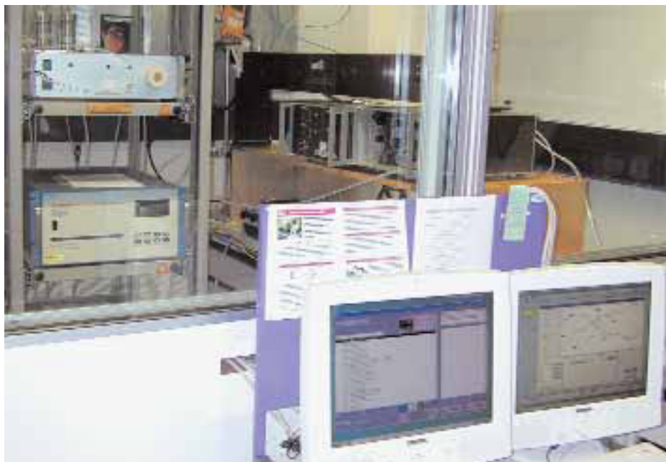
1: METAS ozone laboratory: In the measurement cubicle, ozone reference instruments are calibrated using the primary standard (right). In the foreground the controls for the primary standard and the measurement facility automation.
